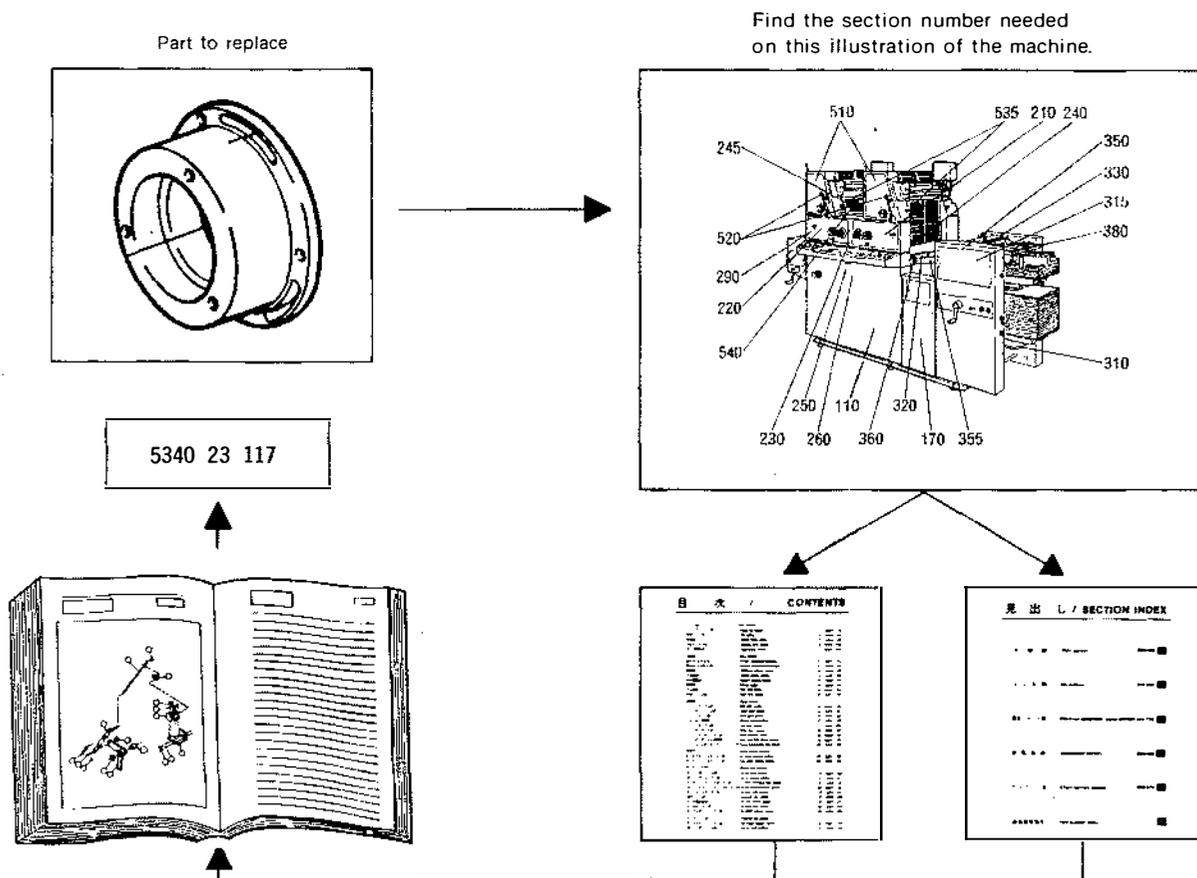
2) To find the section number and the position identification number of the part in the illustration when knowing the part number
